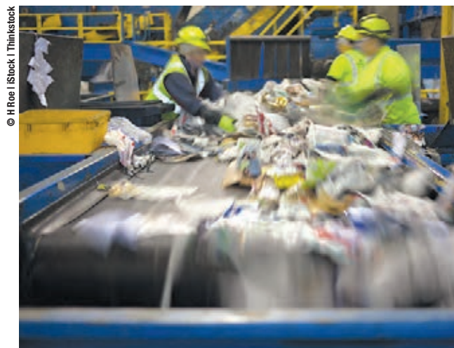
Workers pull recyclables off a moving conveyor belt in a recycling sorting facility. Materials coming into this facility come in as mixed recyclables from “single-stream” carts and bins.
